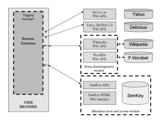
Figure 6: Detailed system modules' architecture.
